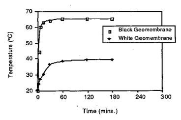
Figure 3.9 - Geomembrane Surface Temperature Differences Between Black and White Colors
