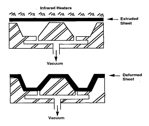
Figure 6.13 - Vacuum Forming System for Fabrication of a Drainage Geocomposite
