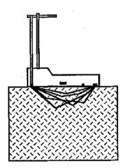
Figure 2.28 - Measurement of Density with Nuclear Device by (a) Direct Transmission and (B) Backscattering
