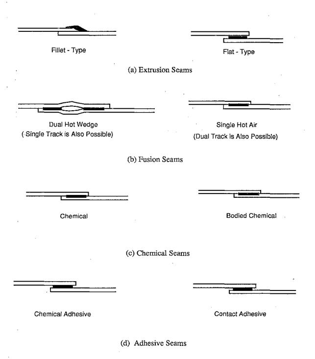
Figure 3.19 - Various Methods Available to Fabricate Geomembrane Seams
