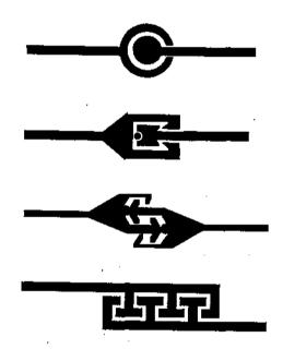
Figure 7.6 - Examples of Interlocks for Geomembrane Walls (Modified from Manassero and Pasqualini, 1992)
