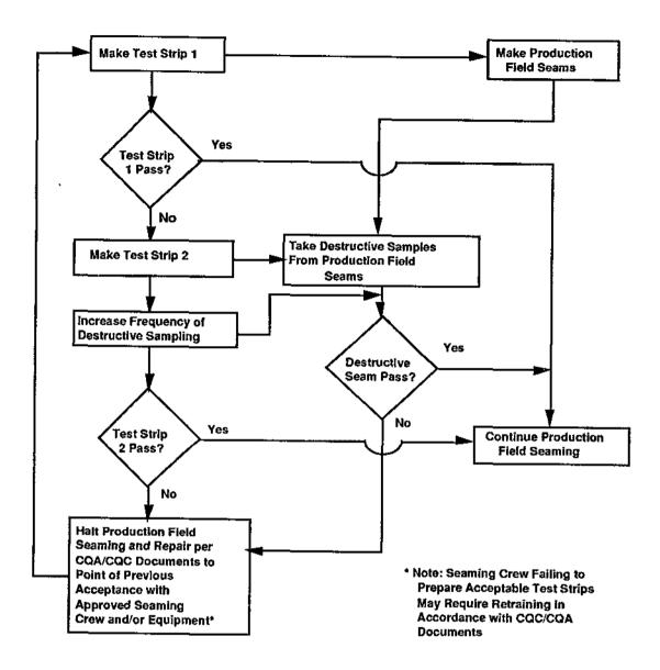
Figure 3.22 - Test Strip Process Flow Chart
