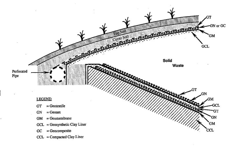
Figure 6.1 - Cross Section of a Landfill Illustrating the Use of Different Geosynthetics Involved in Waste Containment Drainage Systems
