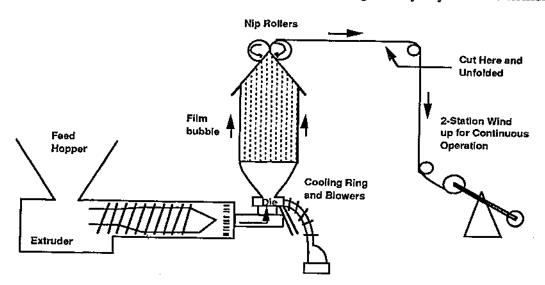
Fig. 3.7(b) - Sketch of Blown Film Manufacturing of Polyethylene Geomembranes
