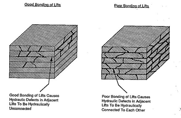
Figure 2.23 - Flow Pathways Created by Poorly Bonded Lifts
