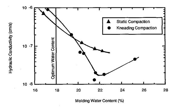
Figure 2.18 - Effect of Type of Compaction on Hydraulic Conductivity (from Mitchell et al., 1965)
