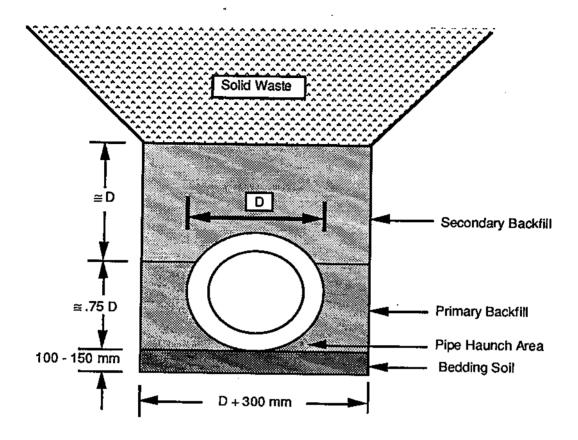
Figure 8.6 - A Possible Buried Pipe Trench Cross Section Scheme Showing Soil Backfill Terminology and Approximate Dimensions (for illustration purposes only).
