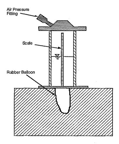
Figure 2.26 - Schematic Diagram of Rubber Balloon Device
