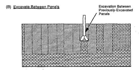
Figure 7.15 - Diaphragm-Wall Construction.
