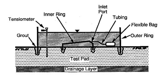
Figure 2.32 - Schematic Diagram of Sealed Double Ring Infiltrometer (SDRI)
