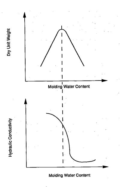
Figure 2.14 - Effect of Molding Water Content on Hydraulic Conductivity
