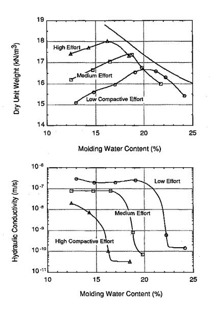
Figure 2.20 - Effect of Compactive Energy on Hydraulic Conductivity (after Mitchell et al., 1965)
