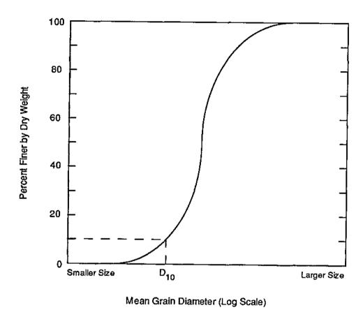
Figure 5.1 - Grain Size Distribution Curve
