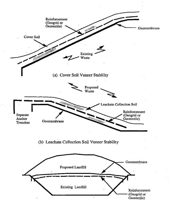
(c) Liner System Reinforcement for "Piggy backing"
