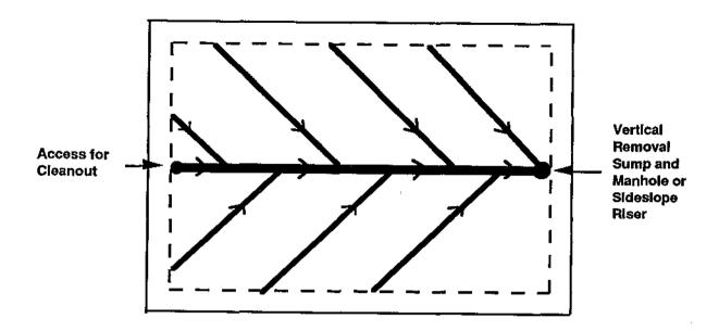
Figure 8.2 - Plan View of a Possible Removal Pipe Scheme in a Primary Leachate Collection and Removal System (for illustration purposes only).
