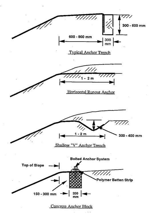
Figure 8.9 - Various Types of Geomembrane Anchors Trenches (Dimensions are Typical and for Example Only).
