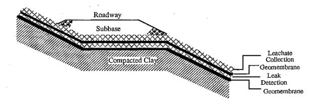
(b) Cross Section of Ramp Roadway
