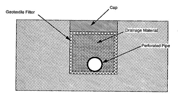
Figure 5.3 - Typical Design of a Drainage Trench
