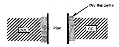
(b) Compacted Clay Liner (CCL) Penetration
