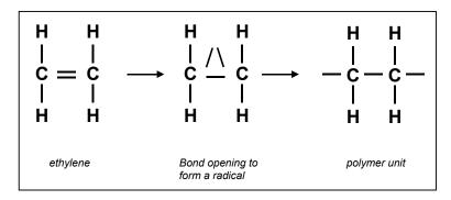
Figure 1 Schematic diagram of the formation of polyethylene.
