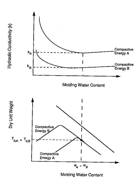
Figure 2.21 - Illustration of Why Dry Unit Weight Is a Poor Indicator of Hydraulic Conductivity for Soil Compacted Wet of Optimum
